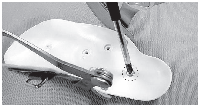
Fig.17 Attachment of SUS Round flat-head screw M4×5 (M4×4 for Small size) 1
