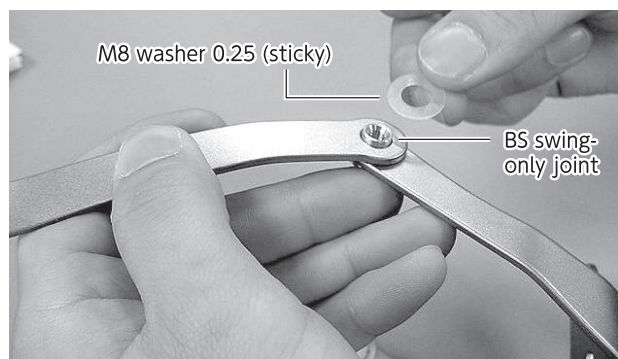
Fig.9 Application of M8 washer 0.25 (sticky)
