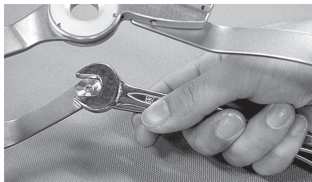
Fig.13 Holding BS swing-only joint
