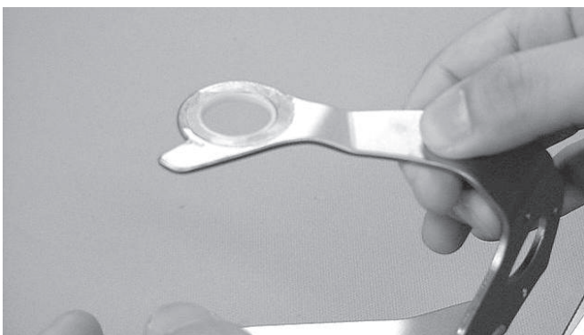
Fig.4 Application of Washer for pivot axis
