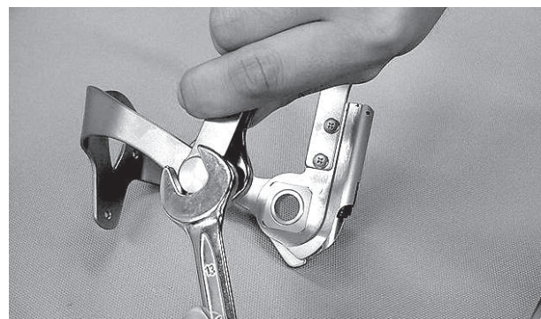
Fig.14 Tightening AL swing-only joint
