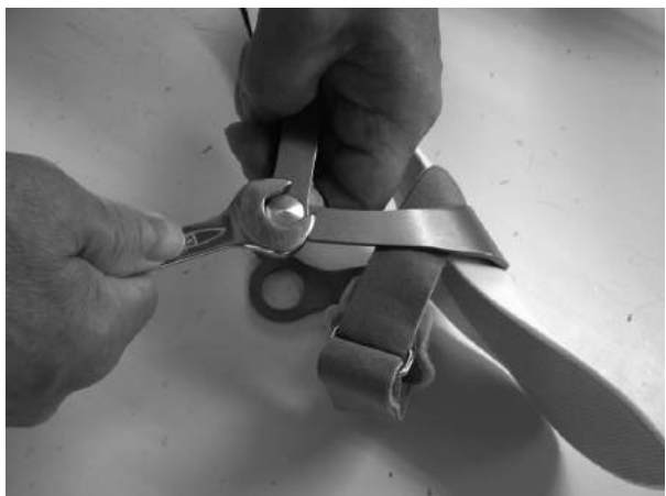
Fig 9 Removal by Spanner
