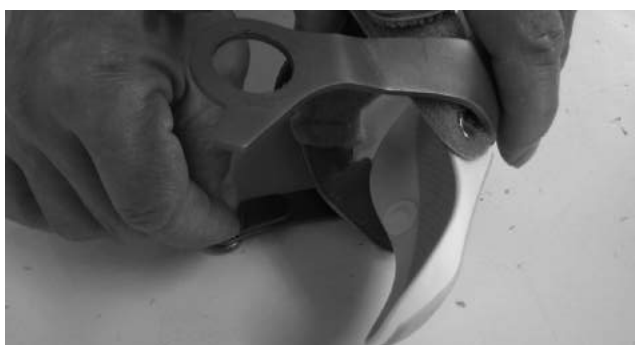
Fig.25 Sticking protection seals
