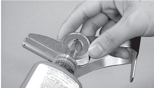
Fig.6 Attachment of Rectangular pivot axis/ Application of Screw locking agent
