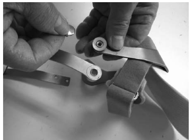
Fig. 10 Removal of Swing only axis
