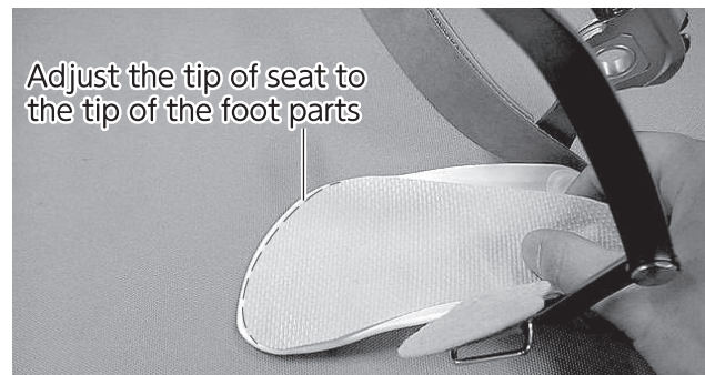
Fig.24 Sticking planter foot seat (Match the toes)
